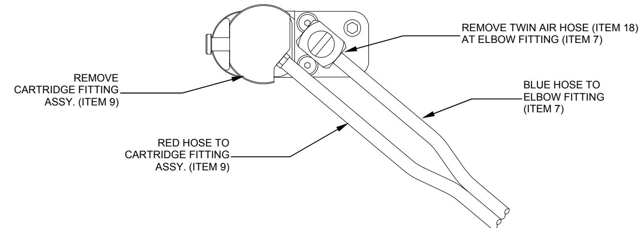
2. Remove the *cartridge fitting assembly* (Item 9) from the *inker assembly*. Inspect the *cartridge fitting assembly* (Item 9) for ink contamination or damage. Clean *cartridge fitting assembly* (Item 9) as necessary and replace the washer (Item 15).
