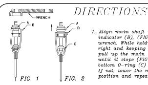
1. Align main shaft indicator (A) with body indicator (B), (FIG. 1) using the plastic wrench. While holding the cartridge upright and keeping the indicators aligned, pull up the main shaft with the wrench until it stops (FIG 2). Make sure the bottom 0-ring (C) has also been raised. If not, lower the main shaft to original position and repeat the above procedure.
