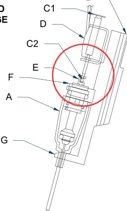
When the cartridge (A) is installed on the holder (B), the plunger (C1-C2) passes through the coil (D) and is captive in the top of the cartridge filament holder (E). Removing the cartridge from the holder with the plunger connected will eventually bend the plunger.
