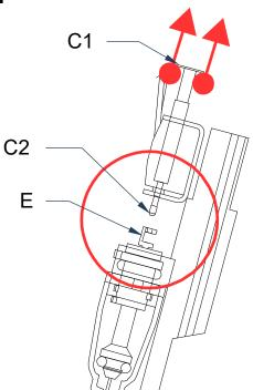
**NOTE:** If Plunger Stop Assembly is installed on the inker, the plunger stop adjustment dial needs to be raised (backed off) until the plunger top (C1) can be lifted enough to disconnect the plunger tip (C2) from the cartridge filament holder (E).
