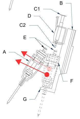
Once the plunger tip (C2) and the filament holder (E) are separated, remove the bottom of the cartridge (A) from the holder dovetail (G) at the bottom of the holder.
