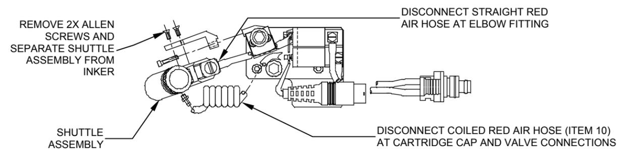
1. Remove the ink cartridge (if installed). Remove the Inker Assembly from the Prober. Retain all inker mounting screws.
