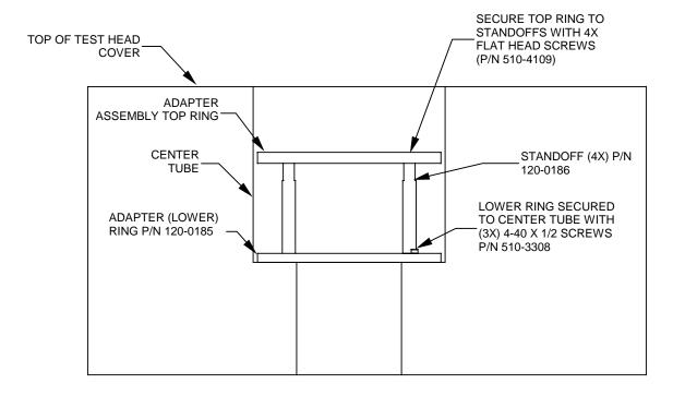
Cutaway view of adapter assembly installation
