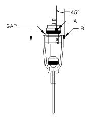
Visually inspect the primed cartridge before installing it on the inker and verify that the following conditions exist;
