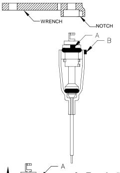
A plastic wrench is used to open and prime a cartridge. The wrench fits very tightly and has a shallow cup with a notch to fit over the top of the main shaft. The notch location is indicated by an alignment "bump" on the end of the wrench.
