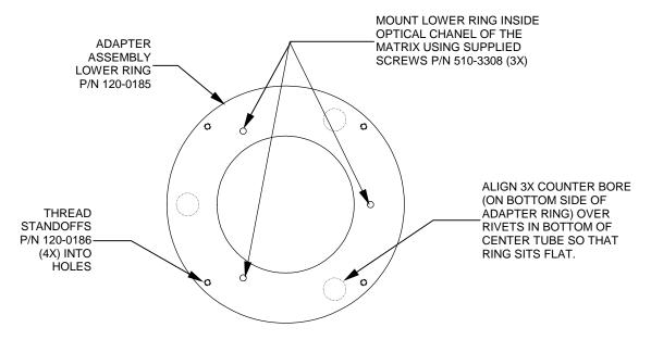
Adapter Assembly Lower Ring, Note counter bore features (3x, far side).
