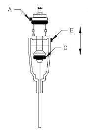
The purpose of priming the cartridge is to insure that the lower reservoir and the *ink flow channels* below the *bottom O-ring* are completely filled with ink. This will insure even, continuous ink flow. To prime the cartridge follow the steps below.
