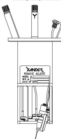
The EG3313 Electric Remote Adjust is an in-line inker that incorporates easy installation and removal from the tester with the added ability to change ink cartridges without undocking the test head. Precise X, Y, and Z adjustments to the inker are possible while the test head is docked and the microscope is in position.
